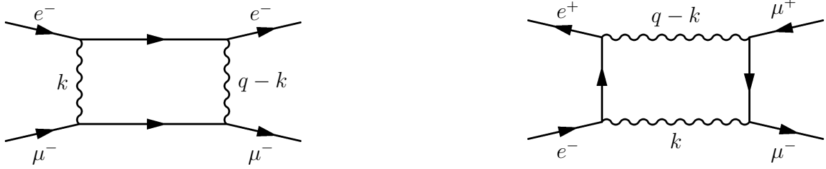
Figure 7.1: Higher order box diagrams with two photon exchange. Left: e^- \mu^- \rightarrow e^- \mu^- scattering. Right: e^+ e^- \rightarrow \mu^+ \mu^- .
